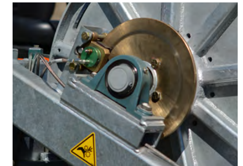
Braking System with Electric-Over-Hydraulic Activation
