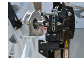
Cab-operated, 16-inch Payout Brake
