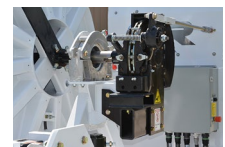
Spider® Pilot Line System with independent levelwind
