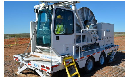
P-2000X Puller featuring the Safe-Zone® Cab
