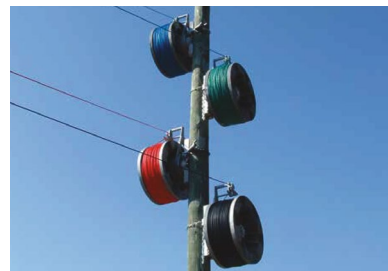
Spider Storage Reel Assemblies with Rope mounted to a pole
