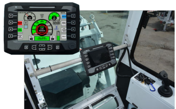
PTX-3500 Control Panel
