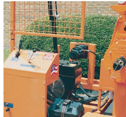
Rear Mounted Control Panel
