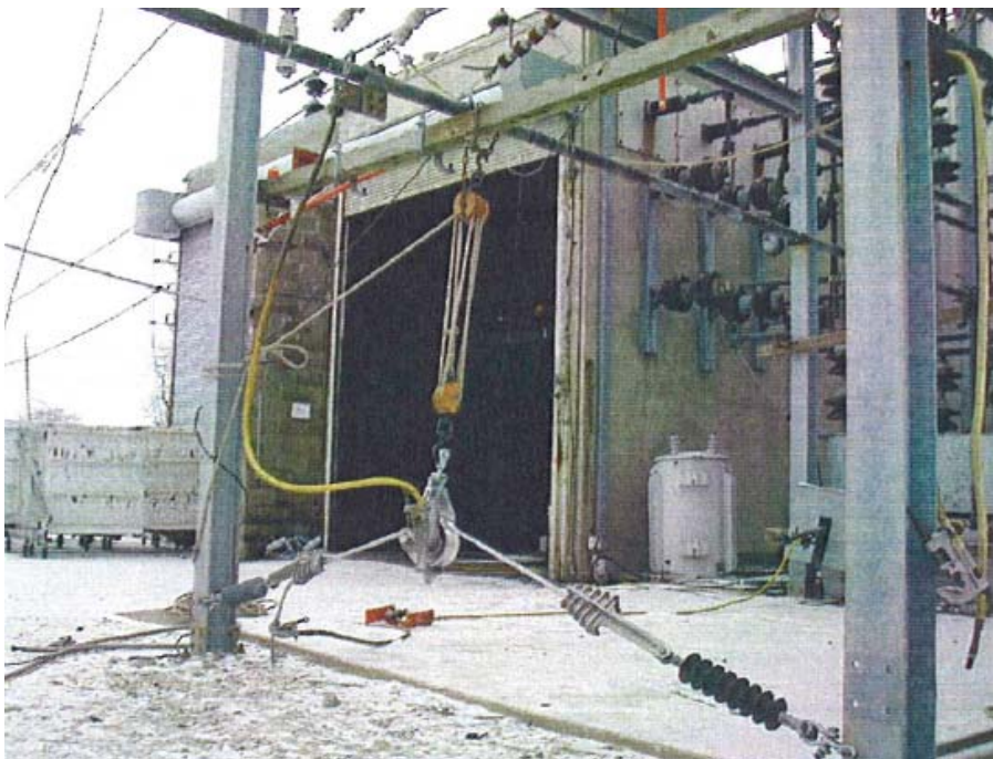
Results of High Current Tests on Sherman & Reilly Model GS-100 Grounding Stud
