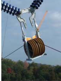
32 inch 7060-U Bundle Block, with HWA-70
