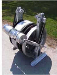
28 inch 7032-FF-L Off-Set Bundle Block, with Block Ground
