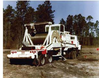
SRU Model DP-300-1 Single Drum Puller 30,000 lbs. with 27,500 ft. 3/4" Swaged Rope
