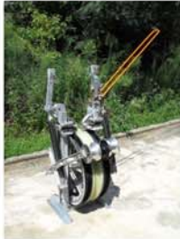
32 inch 7032-NUN-B "Slim Line" Bundle Block, with HWA-70 and Block Ground
