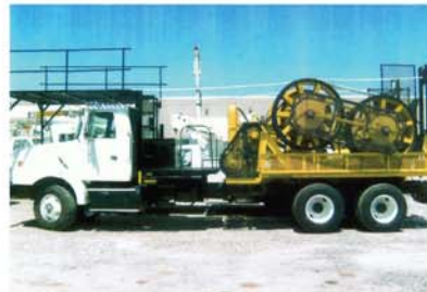
SRU Model BWT-200-60 Bullwheel Tensioner 2-Conductor with 60" Diameter Bullwheel
