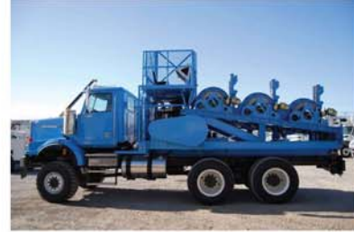
Model SRU-DP-50-3 Drum Puller with 3 x 25,000 ft. 3/8" Swaged Rope
