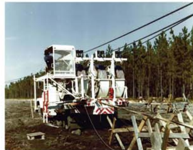
SRU Model BWT-300-72 Bullwheel Tensioner 3-Conductor with 72" Diameter Bullwheel
